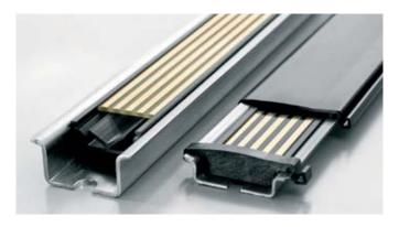
The resistant gold-plated contacts ensure a permanent and reliable contact. The ACT20M modules are simply snapped onto the mounting rail and are automatically in contact with the DIN rail bus. The supply of 24 V DC to the power rail can be from any one of the auxiliary powered ACT20M modules, when that module is itself externally supplied. This allows the rail to power up to 8 other modules (approximately 400 mA). For powering additional ACT20Ms, a separate Feed-In module can be used.
