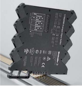
Weidmüller offers a compact and narrow 6mm feed-in module as an alternative. This wires the terminal level directly to the DIN rail bus. Up to 80 modules can be fed with a maximum available current of 2.5 A.
