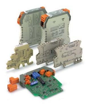
**2-way isolation** separates the signals from each other electrically and decouples the measuring circuits. Potential differences – caused by long line lengths and common reference points – are eliminated. Furthermore, the electrical separation protects against irreparable damage caused by overvoltages as well as inductive and capacitive interference.
